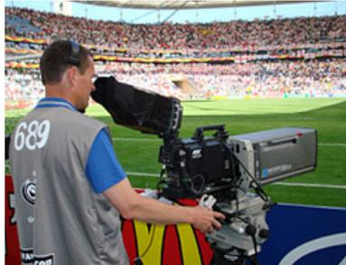
With the capability of recording up to 300 fps, the Hi-Motion is ideal for slow-motion playback for broadcast sporting events.
