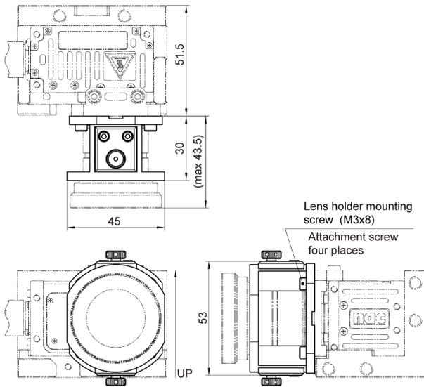
C-Cam Straight figure of mounting 1
