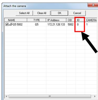
4 A window is shown where it is possible to confirm the contents previously set to the Q5 and the currently connected camera heads.
