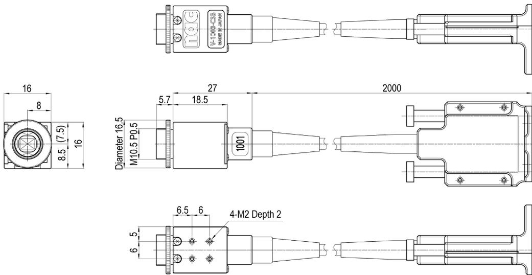
■  $\mu$ -Cam Camera Head Mounting Plate (Straight, Camera Head Attachment)
