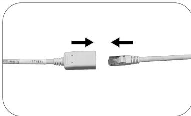
1 Connect an Ethernet cable to the Ethernet connector of the Q-CAM cable. Connect a Windows PC
