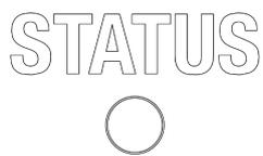
Normally not lit. After connecting the Q-HUB to a power source and pressing the status check button, the battery status can be confirmed.
