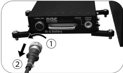
**6** Remove the cable from the 24V Hi-G battery
