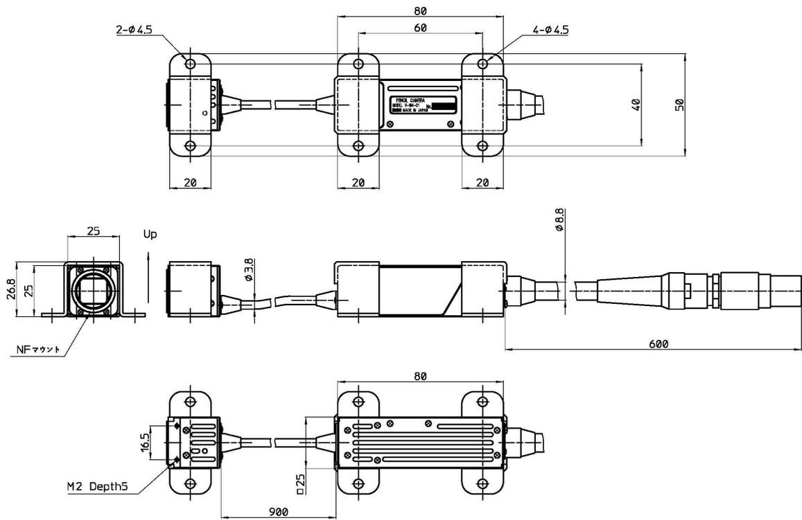
■ S2-Cam Side Type (when using mounting fittings)
