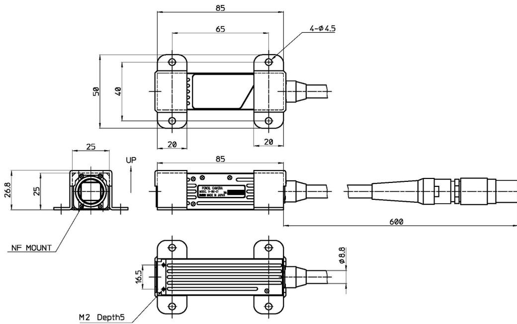
■ P2-Cam SA Type (when using mounting fittings)
