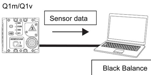
Reads the sensor data from the Q1m/Q1v and produces black balance (corrected data) during PC control.
