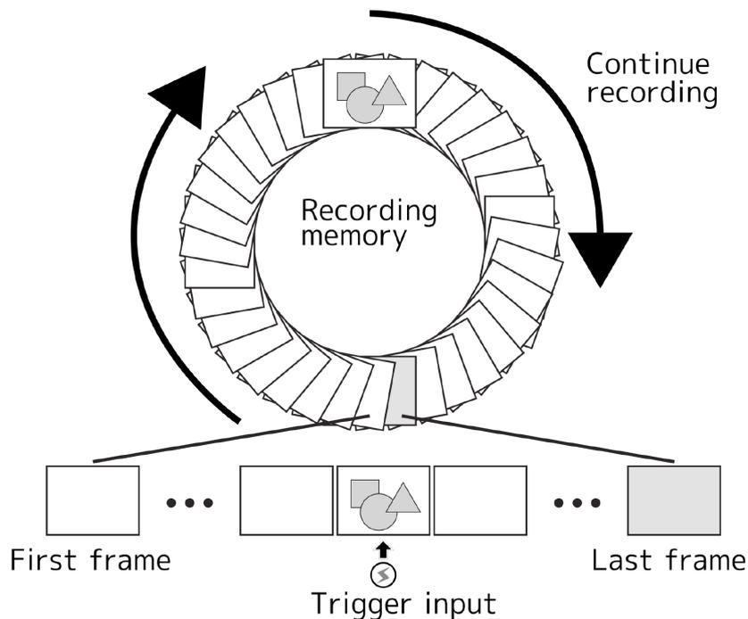
This operation continues until the trigger is input, when the overwrite recording is stopped according to the trigger input and trigger timing settings.
