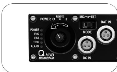
2 Turn the Q-HUB power switch in the direction of the arrow to turn OFF.
