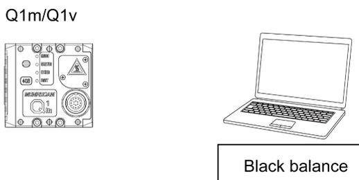
Even if disconnected from the Q1m/Q1v, the black balance obtained is saved in the control PC.
