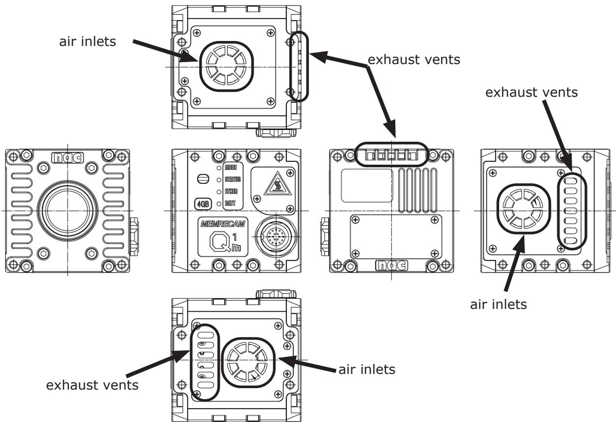
Arrows indicate air inlets and exhaust vents
