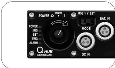
Turn the power switch for the Q-HUB in the direction of the arrow to turn ON.
