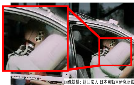
Video at the instant of the crash Since the dummy has leaned forward, part of the head is hidden and cannot be tracked
