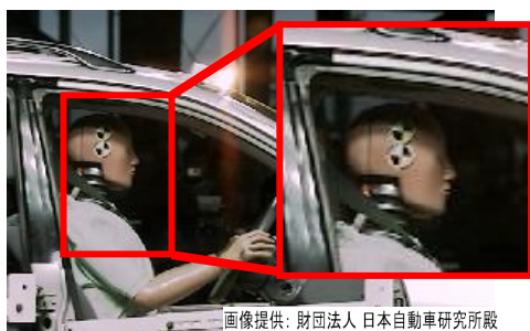
On-board dummy Tracks the outline of the head
