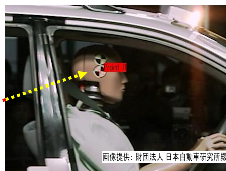
Video at the instant of the crash Since the dummy has leaned forward, part of the head is hidden and cannot be tracked
