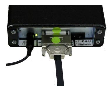
Connect one end (HSSDC Connector) of the Fibre Channel Cable to the PCI card. The release tab should face up. Connect the other HSSDC connector to the *MEMRECAM* fx camera. <u>Do not power up the</u> <u>MEMRECAM fx camera at this time.</u>
