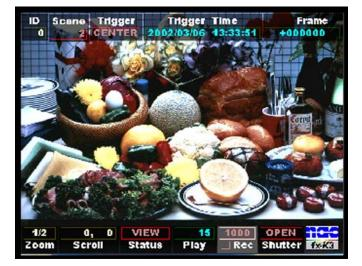
To modify the record settings select the **Rec** box using the **LEFT/RIGHT** keys while in **VIEW** mode.
