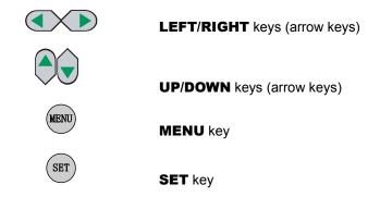
The IBOX display boxes are accessed by using the **LEFT/RIGHT** keys while in **READY** or **VIEW** modes. Once the particular box is selected, use either of the following methods to change the settings,
