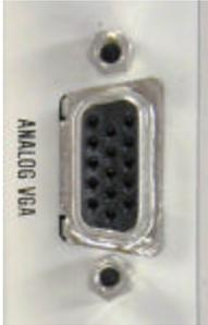
Connect to the analog VGA multiscan monitor
