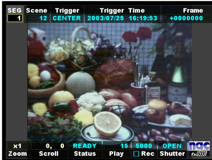
5) In the segment IBOX, pressing the **SET** key enters the segment changing mode (the segment number indication box turns black).
