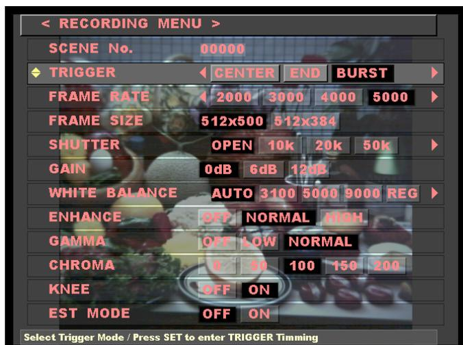
■ Selection of burst recording mode using IBOX
