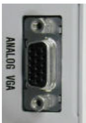
Connect to the analog VGA multiscan monitor
