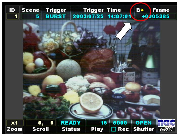
When the burst-recorded image is to be invoked, press the **TRIGGER** key so that the foremost image in each burst-recorded block is reached.
