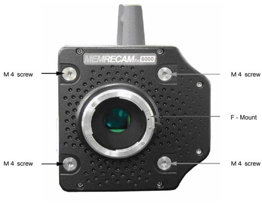
Photo-2 RX Camera Head Front Panel
