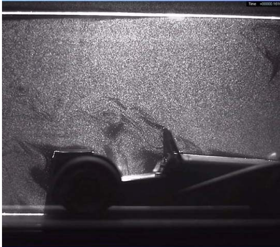
Airflow around a model car - Memrecam GX-ir at 2,000 fps
