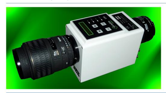
The Invisible® Vision UVi series of camera accessory intensifiers are designed to add low light, extended spectral range (from UV to NIR) and fast gating in a compact and all inclusive, easy to use lens coupled package. Typical applications are in combustion, electric discharge, biomedical and ultra-high speed stroboscopic or shuttering techniques with high speed or conventional video cameras.
