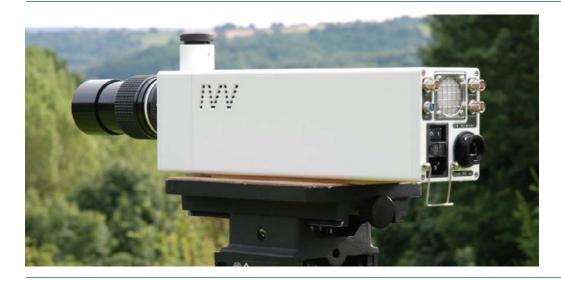
he Invisible® Vision PiV series of multi-frame cameras are designed to achieve ultra fast shuttering combined with zero frame to frame distortion - so essential for quantitative particle image velociometry applications in the analysis and scientific modelling of high speed events.
