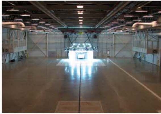
LEFT: The KHS lighting system boasts 28 4,000W units, which are rail-mounted for easy transition from frontal to side crash scenarios
