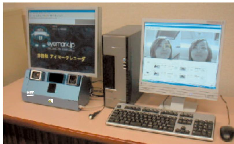
**100% Contact-free, thus an examinee does not wear any special device (helmet, headband, glasses, and others) for measurements. NAC EMR-AT VOXER allows users to track gaze position on monitor/display without any physical contact with the examinee.**
