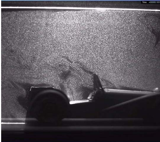
Airflow around a model car - Memrecam GX-ir at 2,000 fps
